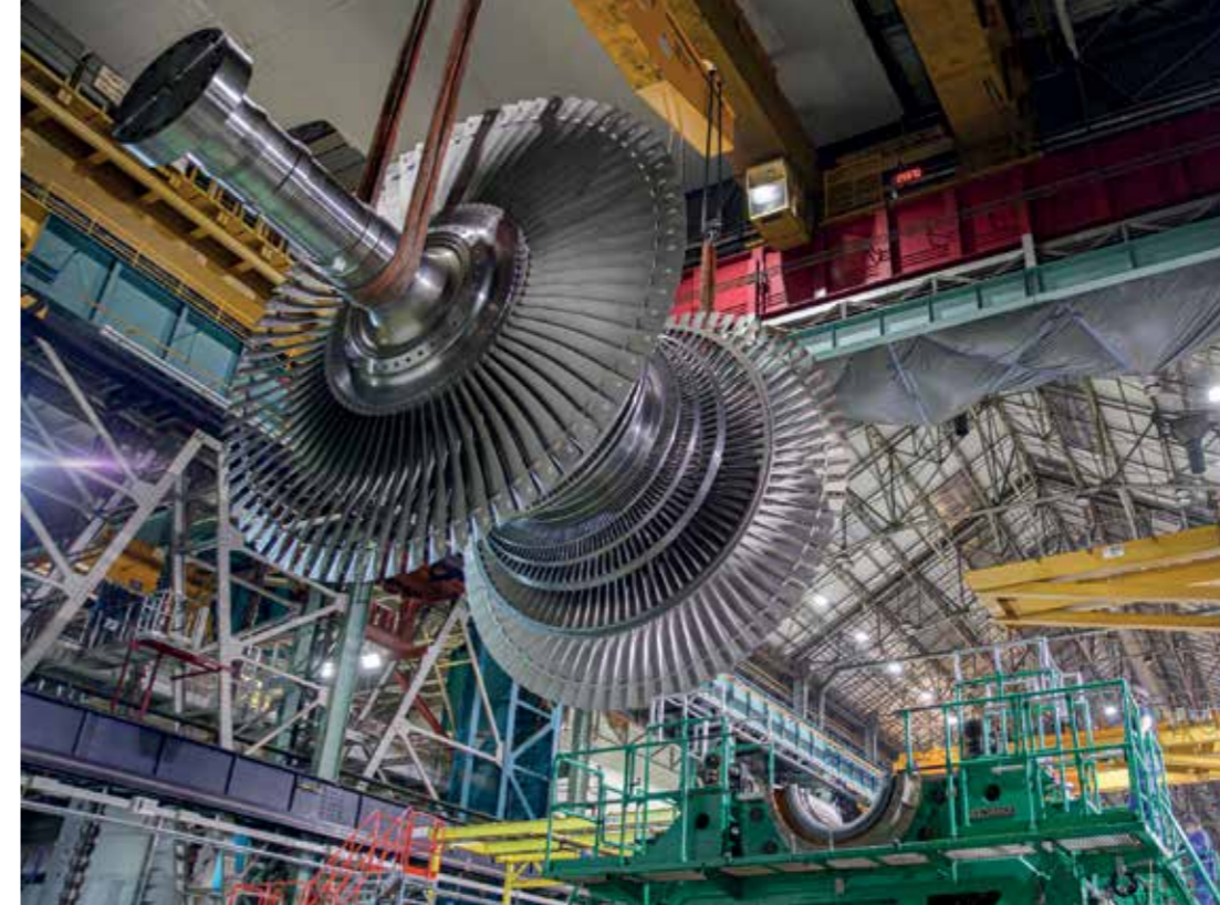
Above: Lift of Arabelle LP rotor at Belfort factory Source: Arabelle Solutions
