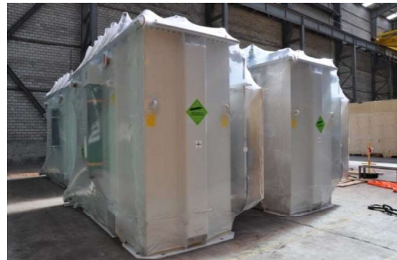
Figure 40: Nitrogen purged transformer furnished with gas cylinder
